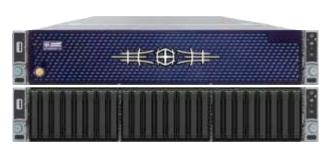
Each AP-3215 platform contains up to 48 cores in dual high-speed Intel Broadwell processors, up to 1.5TB RAM, two built-in 10GbE ports, and a high count of external SAS-3 ports for disk access, and a variety of client-facing network interfaces. That's 3TB of RAM and 384Gb total SAS bandwidth in the maximum HA configuration.
