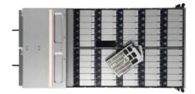
The WARP 38002-H uses the WDS-9460 JBOD to expand the capacity provided within the central storage controller platform. A pair of redundant SAS IO modules per shelf provides up to 384Gbps of SAS throughput from each shelf to each controller. In a full rack, the total available SAS bandwidth can reach 3Tbps.
