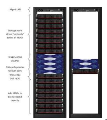
In the simplest configuration, the WARP 41001-M uses the WDS-2224 JBOD to provide capacity provided in a three-chassis "Pod" configuration: 2x OSS heads and one OST JBOD with enterprise SSD modules to achieve maximum write and read performance. Each SSD exceeds 100,000 IOPS per module, making the WARP 41001-M easily capable of 192TB and 1 Million IOPS per OST shelf.
